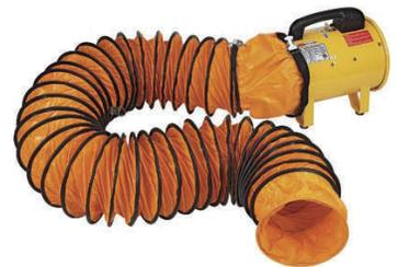
Uninsulated, flexible HVAC duct may be used for ducting the air into and from the workspace as a convenient and inexpensive alternative to the hose assembly pictured above.
